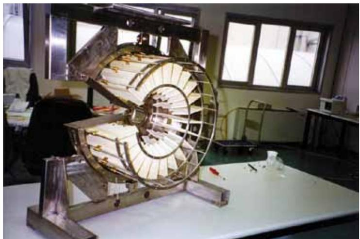
Fig. 26 GARFIELD (General Array for Fragment Identification and Emission of Light particle Dissipative collisions).
