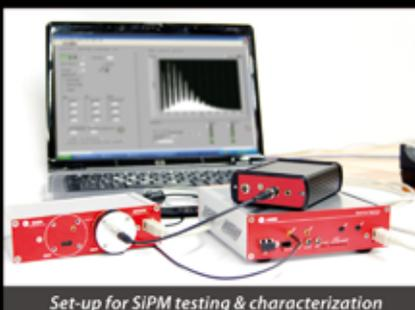
Set-up for SiPM testing & characterization
