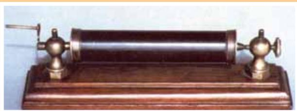
Fig.1 Coherer (*tubetto a limatura*) by T. Calzecchi Onesti (Calzecchi Onesti Family courtesy).
