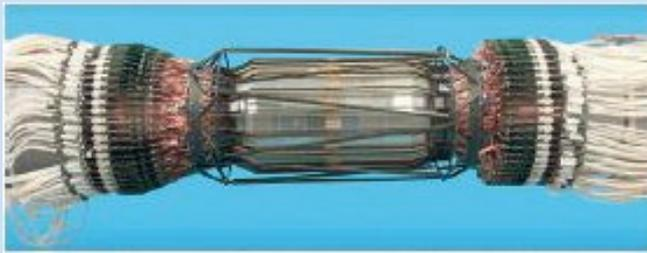
Fig. 17 The BABAR silicon vertex detector made of 5 layers of double-sided strip detector. The shape, lamp-shade-like, allowed a good geometrical acceptance. The sensors were fully designed including the production parameters in the INFN laboratory of Pisa and built full custom in a small foundry.
